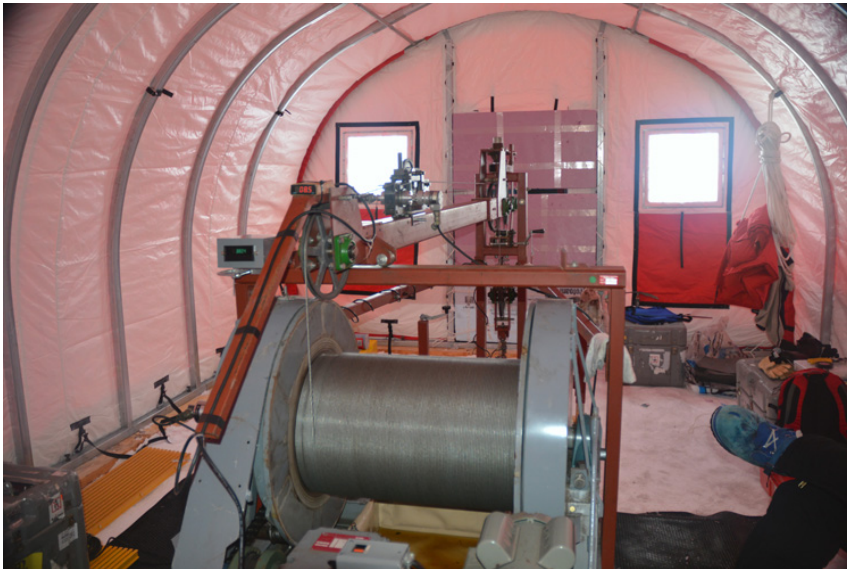
View of the inside of the borehole logging tent and the USGS (now IDDO) Deep Logging Winch. Photo: Don Voigt.
