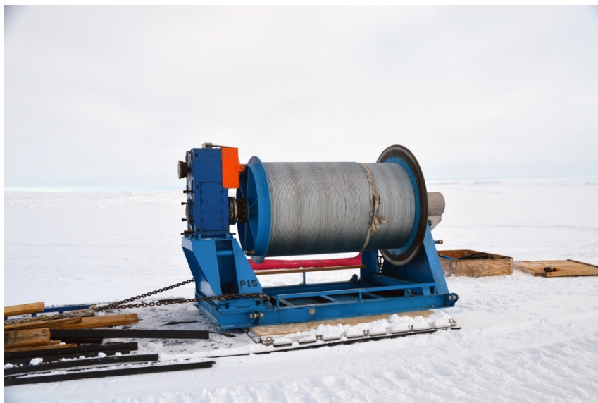
The DISC Drill's winch drum successfully removed from the drilling arch. Photo: Don Voigt.
